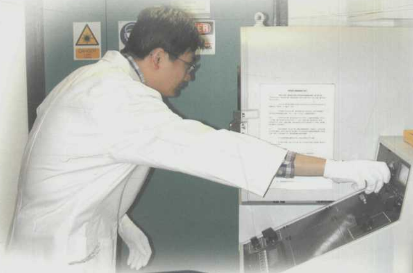
「真空離子鍍膜機」系統有助套取指紋 A fingerprint specialist making use of a "Vacuum Metal Deposition Chamber" to collect fingerprint evidence from exhibits
