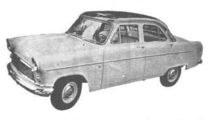
Points of interest. 4 cyl. overhead valves. B.H.P. 59/55, 12 volt lighting system. Can be fitted with tubeless or conventional tyres. Top speed in the region of 79 m.p.h. with a petrol consumption whilst touring about 30 m.p.g.
