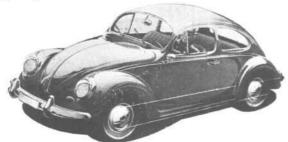
Points of interest. 4 cyl. 1192 c.c. 4 forward gears, syncro. in 2nd, 3rd and top. Fuel tank capacity of  $8\frac{1}{2}$  gallons, and a fuel consumption of around 39 m.p.g. The maximum speed is in the region of 70 m.p.h.
