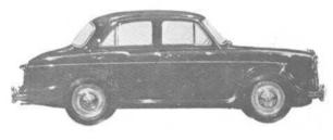
Specifications of interest, 4 Cyl: 1489 c.c. overhead valves, 4 speed gear box with synchromesh on 2nd, 3rd and Top. Lockheed hydraulic fully compensated brakes: overall length 12'8", width 5'2", height 5'0".
