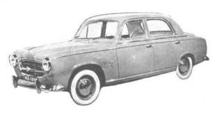
Points of interest. 4 cyl. 1468 c.c. overhead valves, mechanical fuel pump, 12 volt lighting system, turning circle 15 feet 6 inches, length 14 feet 8", width 5'6".
