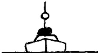
Power driven vessel of less than 65 feet in length under way using combined lantern
