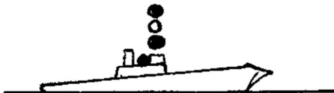
Vessel engaged in laying or in picking up a submarine cable, making way
