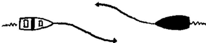
When two power-driven vessels are meeting end on, each shall alter course to starboard (right) so as to pass on the port side of the other.
