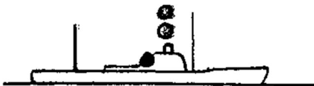
Vessel not under command making way through the water
