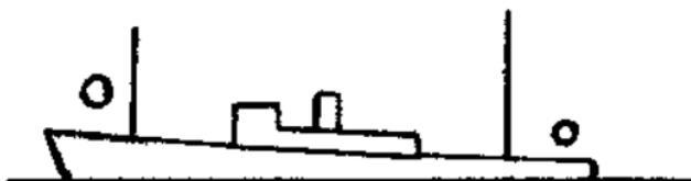
Vessel of 150 feet and over at anchor
