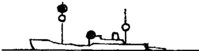
Vessel engaged in trawling showing optional white light, making way
